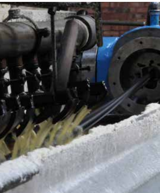
220° salt bath to accelerate the vulcanization process
