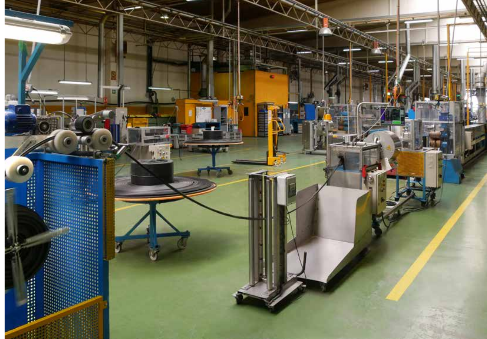
Line end with automatic take-up device
